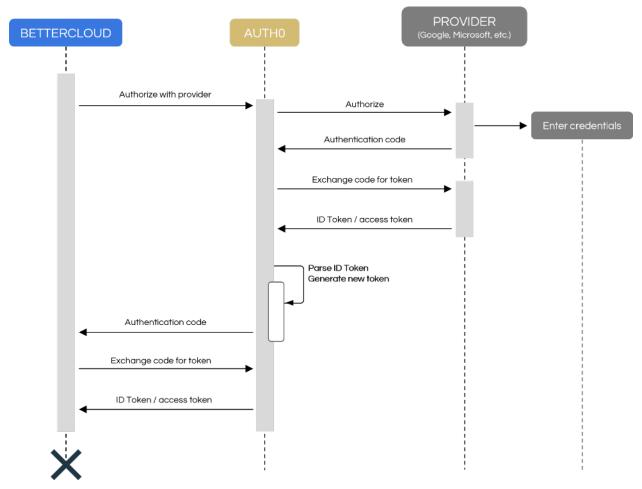
The diagram above illustrates how we use OpenID Connect (OIDC) via Auth0 to authenticate customers to our service and to the SaaS applications they integrate with us.
