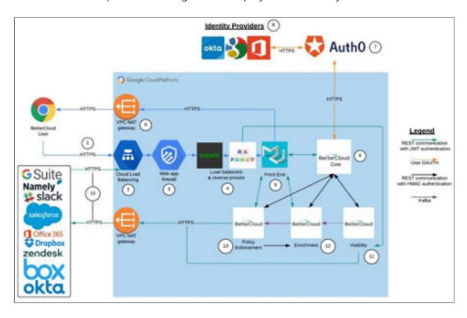
Data flows are generally restricted using Google Compute Engine (GCE) firewalls and supplemented by other technologies illustrated in the diagram, such as NGINX and HAProxy routing rules and the VPC NAT gateway firewall. In GCE, data flows are dropped unless explicitly permitted by a rule. We leverage the default encryption-at-rest provided by GCP, which protects the data on disk with AES-256 or AES-128 encryption. Additional detail below.
